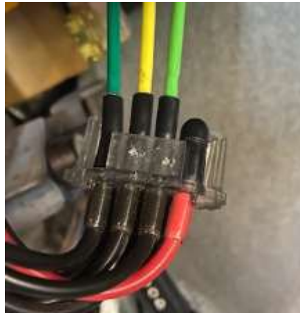
Figure 8: Seven Position Vacuum Line Connector, Red Vacuum Line Side.
