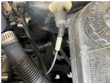
Figure 5: Brake Booster Vacuum Line Connection.
