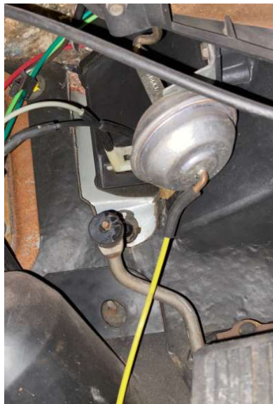
Figure 3: Drivers Side, Lower Vacuum Actuator.
