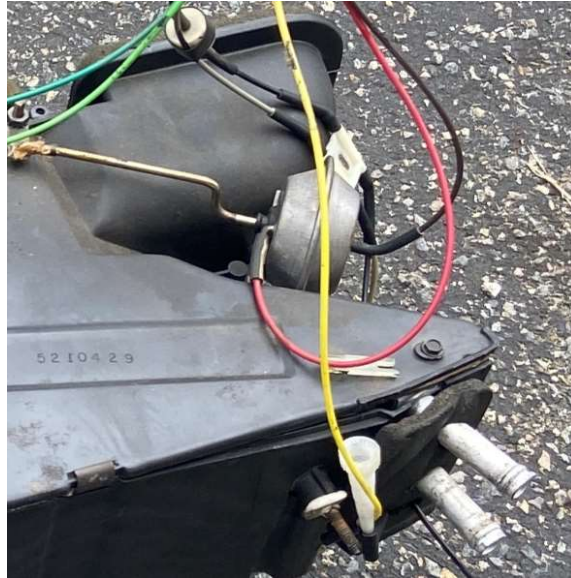
Figure 2: Vacuum Actuator, Drivers side, Top.
