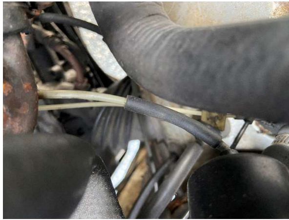
Figure 4: Heater Control Valve Vacuum Line.
