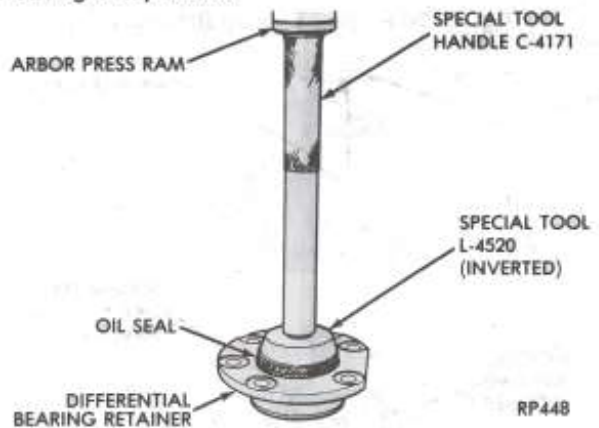
Fig. 2—Install Differential Bearing Retainer Seal
