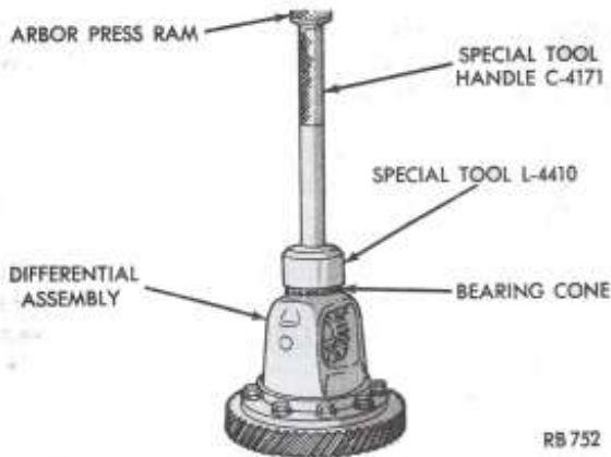
Fig. 2—Install Differential Bearing Cone
