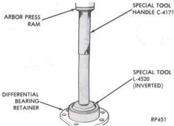
Fig. 5—Install Oil Baffle
